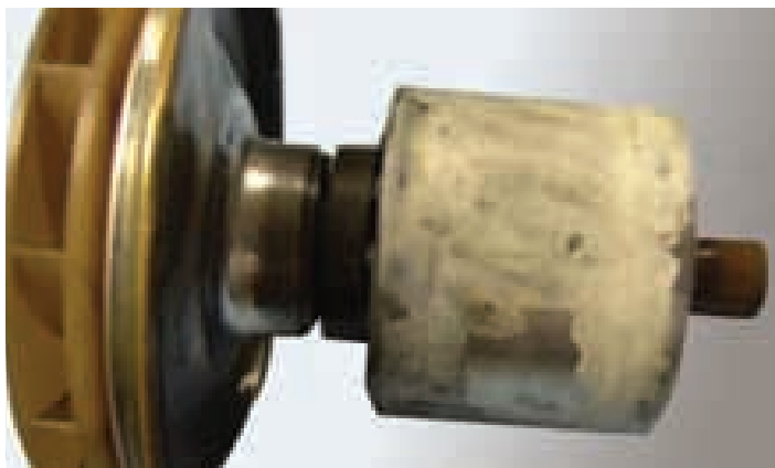
A circulating pump damaged by system debris and pollutants
